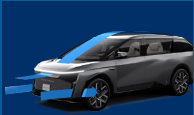
The Model D’s body design incorporates S-ducts and air curtains to reduce aerodynamic drag
